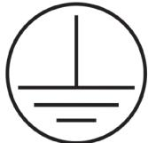
**PROTECTION CLASS 1 - FIXTURE MUST BE PROPERLY GROUNDED.**
