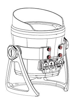
**CLAMP INSTALLATION:** Insert a bolt of appropriate size and rating for the desired clamp through the mounting hole of the clamp, and then insert it through the center hole on the mounting bracket of the fixture. The bolt should pass through both the clamp and the fixture's bracket. Thread a matching washer and locking nut onto the bolt to secure it in place.
