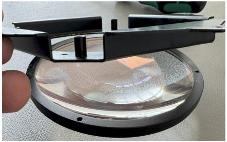
**Step 6:** Realign the holder assembly onto the shutter plate assembly, ensuring the screw posts are aligned over the pressure springs.
