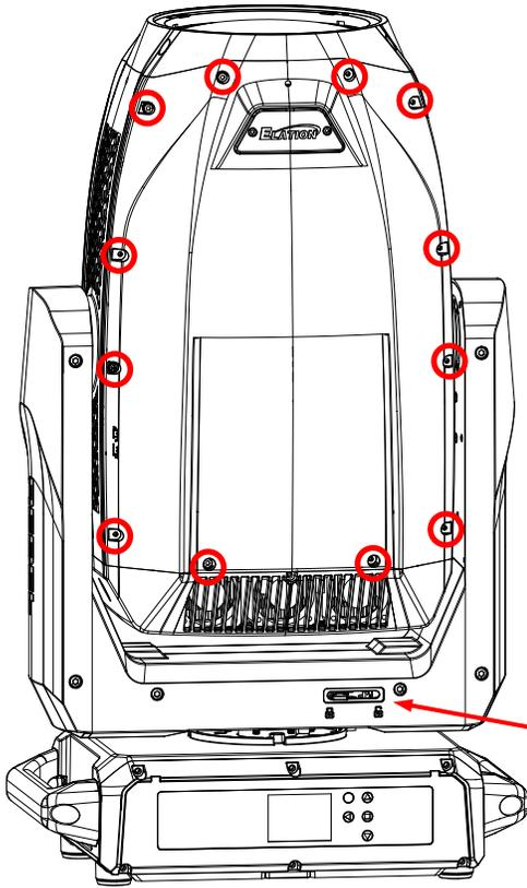
Place the fixture on a firm flat surface. Locate the (12x) hex screws securing the panel on the **Pan Lock** side of the moving head and remove them.
