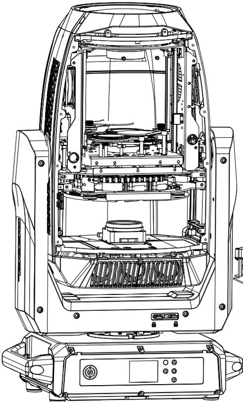
Carefully remove the Rotating Wheel Gobo Assembly Module and set it on a clean surface.
