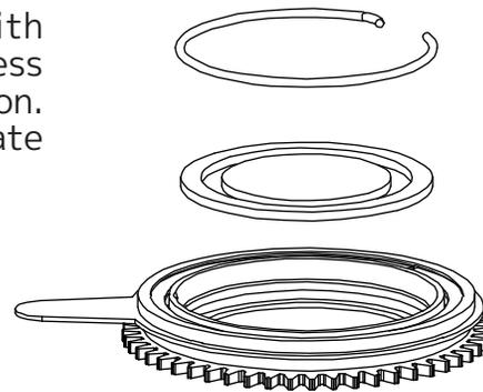
**Note:** To ensure proper Gobo orientation on the Rotating Gobo Wheel, align the Alignment Indices before installing the Retention Spring.
