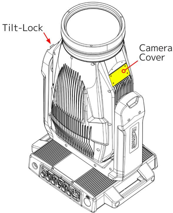
2. Remove (10x) screws indicated in the diagram below from the cover, or proper orientation, note the location of the camera cover, which is opposite of the Tilt-Lock.
