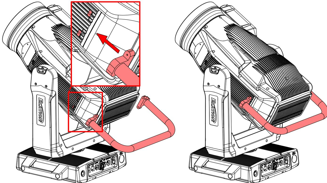
Locate the desired position for attaching the Balance Weight to the Side Handle. Attach the Balance Weight to the Side Handle and secure with thumb screw.
