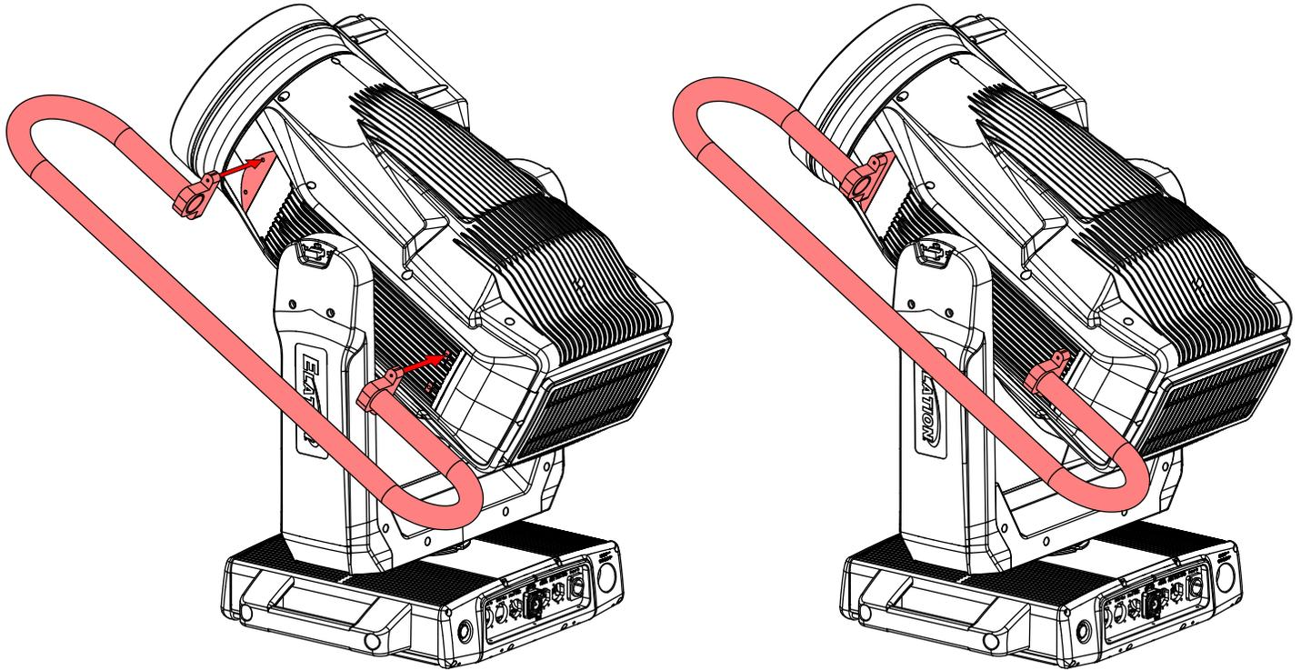
Locate the desired position for attaching the Balance Weight to the Side Handle. Attach the Balance Weight to the Side Handle and secure with thumb screw.
