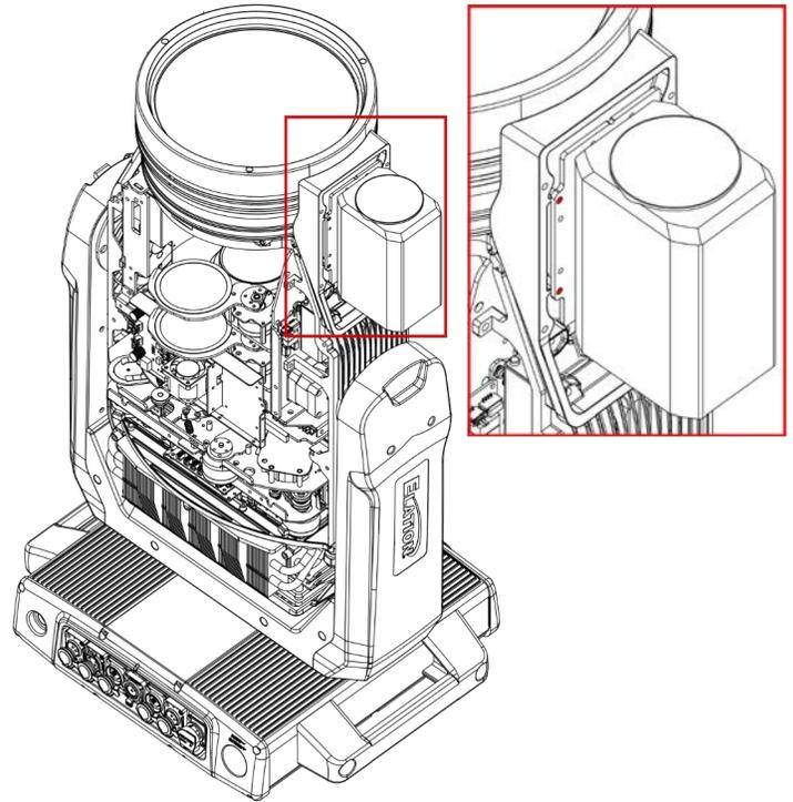
7. Attach the camera cover with (4x) screws on both sides to secure it.
