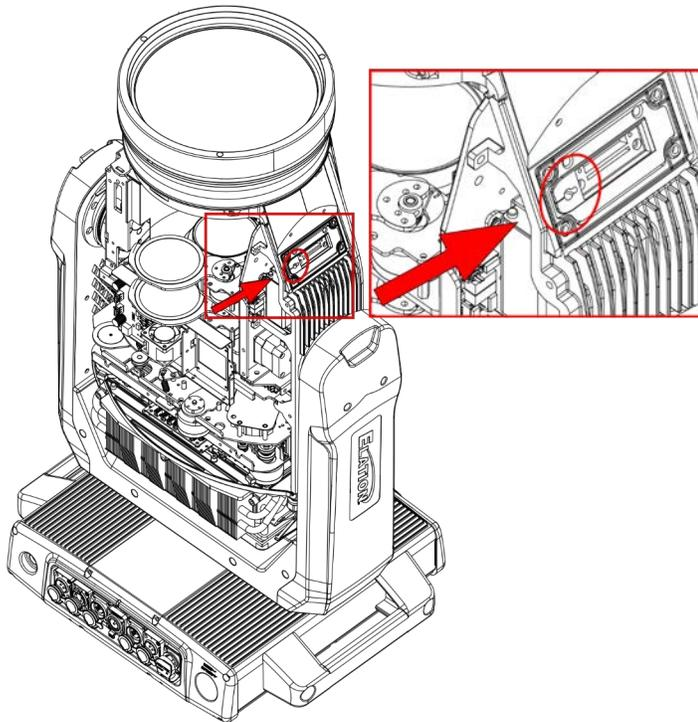
4. Insert the network cable and BNC cable into the designated holes, then flip the reversible rubber stopper back to its original position to secure the cables.
