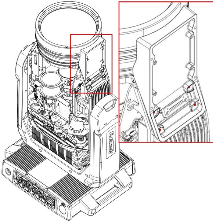
6. Attach the camera to the top of the camera mounting bracket. Secure the camera mounting bracket using four screws on both sides, then connect the network port and BNC interface.
