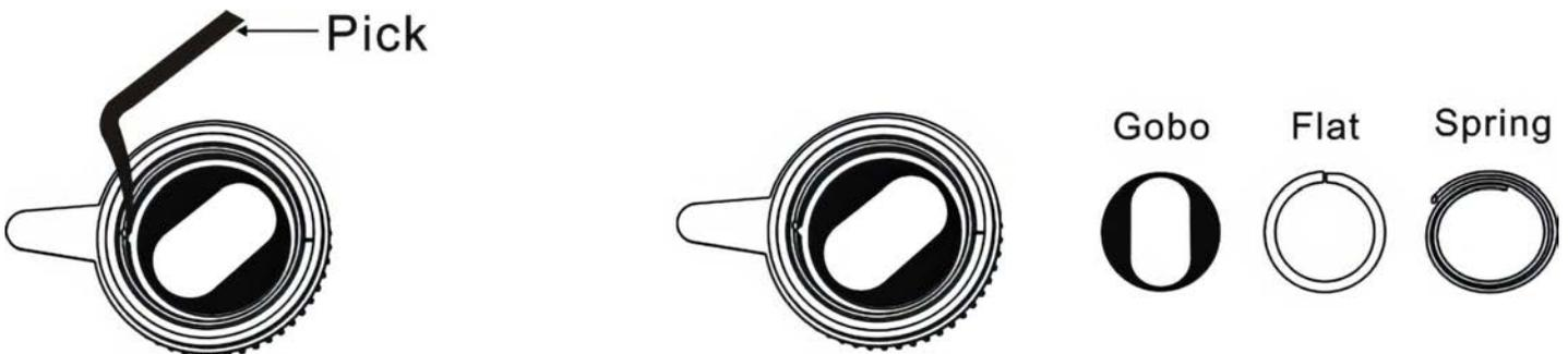
Locate the tab of the spring, and with a precision pick (or similar tool), carefully press the retaining spring inward to relieve the tension. Remove the retaining spring and carefully separate the GOBO from the GOBO Holder. Lastly, remove the flat washer attached to the removed GOBO and attach it to the desired replacement GOBO. Install the replacement Rotating GOBO following the steps above in reverse order.
