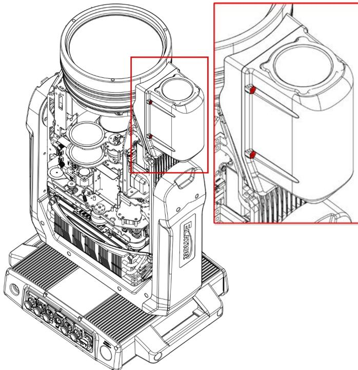
8. Attach the front light cover with screws to secure it and complete the camera installation.
