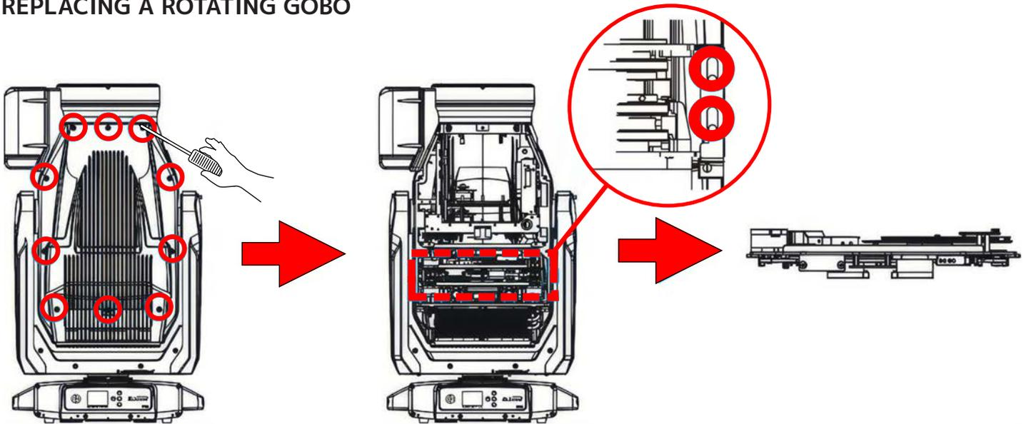
Place the Elation Proteus Brutus FS fixture on a firm flat surface. Locate the (10x) screws on the side of the moving head and remove them. With the panel set aside, locate the Gobo Module Assembly and remove the (4x) screws that secure it to the internal housing frame.
