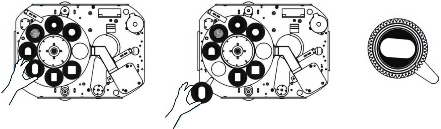
Locate the specific Rotating Gobo to replace. Carefully grip the Gobo using your thumb and index finger, gently lift it slightly, and then pull it out and away until it fully clears the Gobo Wheel.
