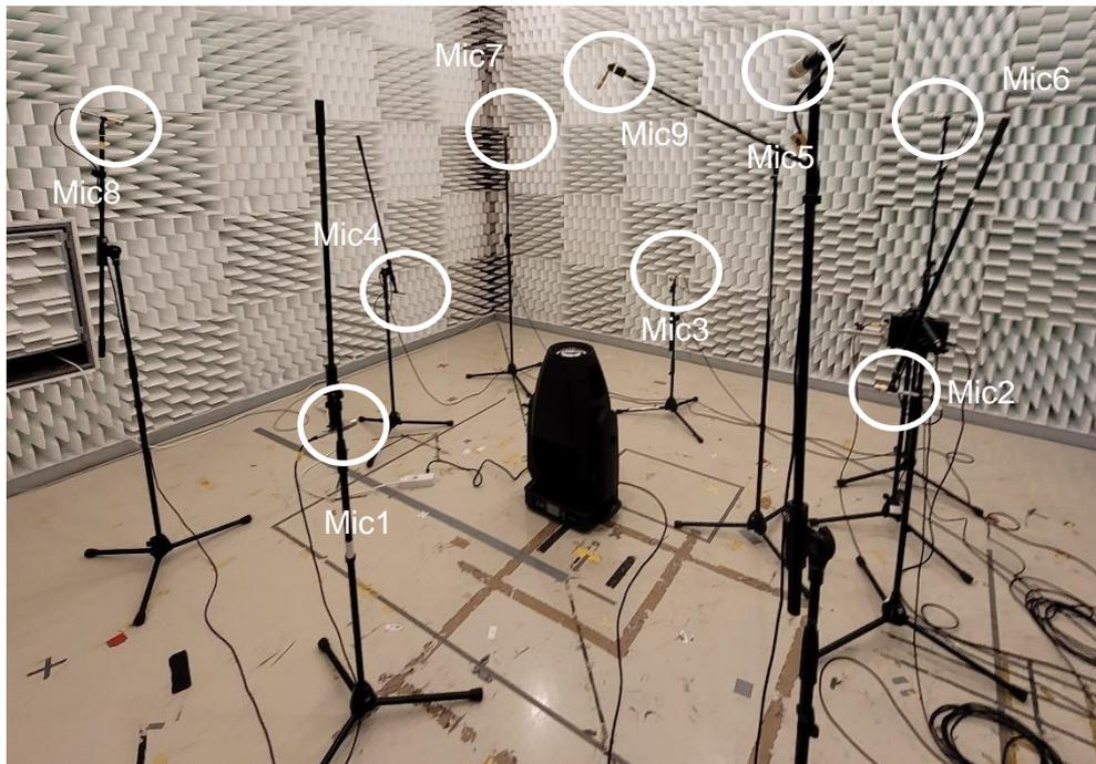
Figure 1. Semi-anechoic measurement room, the device under test (here Elation FUZE TEATRO) and the nine microphone positions.
