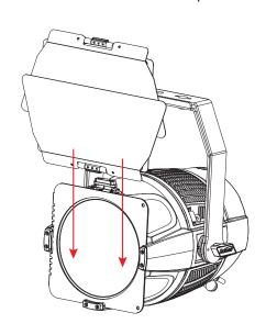
3. If the fixture is being installed in an overhead location, such as hanging from a truss, the barndoors must be secured with their own independent safety cable. The safety cable attachment points can be found at the base of the barndoor unit near where it comes into contact with the fixture. Additionally, always orient the unit with the gel frame latch facing upwards, so that the accessories will not fall in the event that the latch fails.
