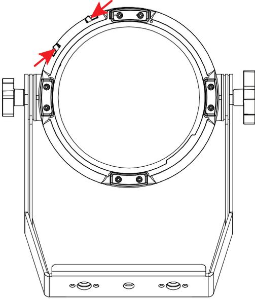
2. Insert the optional lens into position on top of the forward face of the fixture, then release the latches to fix in place.
