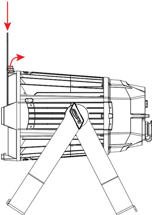
2. Slide the barndoor into the slot in front of the gel frame, then close the gel frame latch to secure in place.
