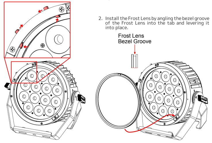
3. With the Frost Lens installed, slide levers outward to lock it in place.
