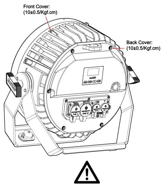
CAUTION! DO NOT OVER TORQUE SCREWS AS THIS CAN CAUSE LEAKAGE ISSUES! TO CONFIRM THE IP65 INTEGRITY, TEST FIXTURE USING THE ELATION IP TESTER. CONTACT ELATION SERVICE FOR MORE DETAILS.
