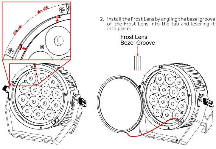
3. With the Frost Lens installed, slide levers outward to lock it in place.
