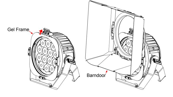
3. Return the retaining clip to the original position to lock the barndoor in place.
