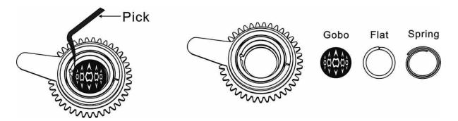
Locate the tab of the spring, and with a precision pick (or similar tool), carefully press the retaining spring inward to relieve the tension. Remove the retaining spring and carefully separate the GOBO from the GOBO Holder. Lastly, remove the flat washer attached to the removed GOBO and attach it to the desired replacement GOBO. Install the replacemet Rotating GOBO following the steps above in reverse order.
