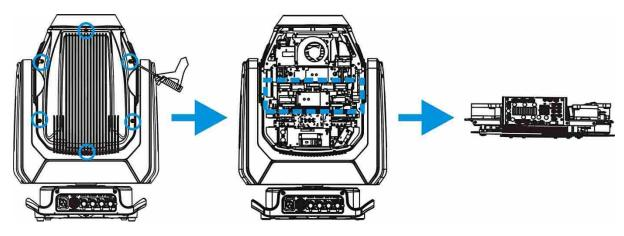
Place the fixture on a firm flat surface. Locate the (6x) screws on the side of the moving head and remove them. With the panel set aside, locate the Pattern Bracket Assembly and remove the (4x) screws that secure it to the internal housing frame.
