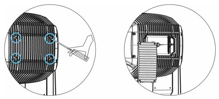
4. Loosen the two slotted thumb screws, and unclip the bottom panel safety cable, and remove the lamp socket cover, exposing the lamp socket.
