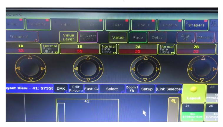
2. When fine-tuning of the barndoors is required, place the unit on a table and set the tilt to a value of 128. On your console, set all 4 barndoor blades to a value of 55, so that the barndoors display the position as shown in the pictures below.
