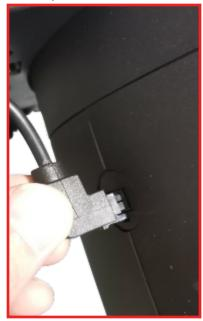
6. To disconnect the Power/ Data Connector, depress the toggle-lock to disengage it, and with a firm grasp of the connector body, pull connector straight from socket. Follow steps in reverse order to remove the Barndoor.
