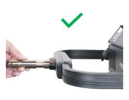
2. Locate the notched face of the junior pin and hold it against the clamp mounting point located on the top side of the yoke. The notched surface of the junior pin must sit flush against the matching groove on the surface of the clamp mounting point.
