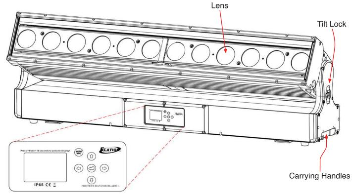
LCD Display & System Menu Controls
