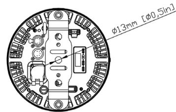
**DIMENSIONAL DRAWINGS (YOKE BRACKET ATTACHED)**
