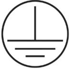
**PROTECTION CLASS 1-FIXTURE MUST BE PROPERLY GROUNDED.**
