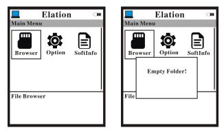
Note that out of the box, the MicroSD card is blank. Make sure the MicroSD is inserted, then select Browser and press ENTER. The message "Empty Folder!" will be displayed.
