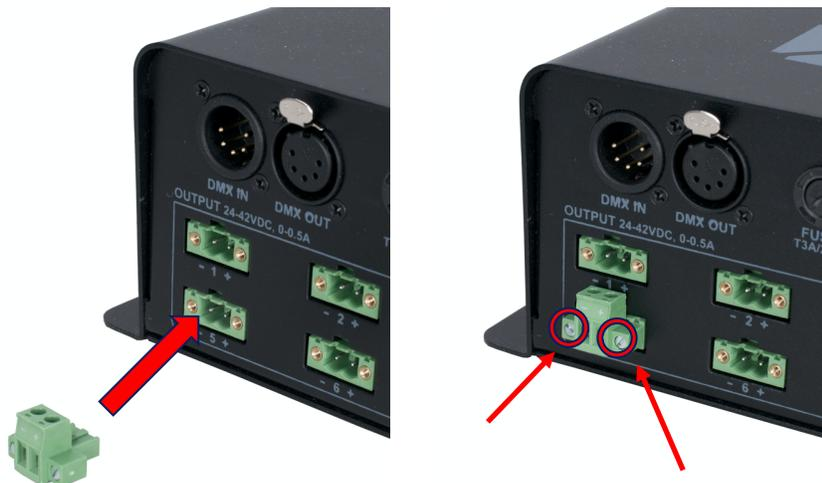
Begin by inserting the male end of the Phoenix connector into the desired signal output port on the driver, making sure that the latch on the Phoenix connector engages with the signal output port. Tighten the two screws located to each side of the wire terminals, as highlighted in the image to the above right.
