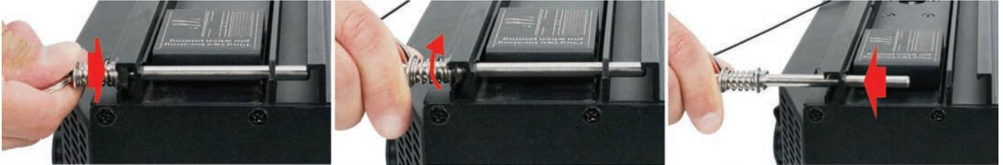
1. To remove spring-loaded locking-pin, compress the spring enough to clear the rail, rotate ring to vertical orientation (stepped rail-block to a horizontal orientation), and pull pin straight out.
