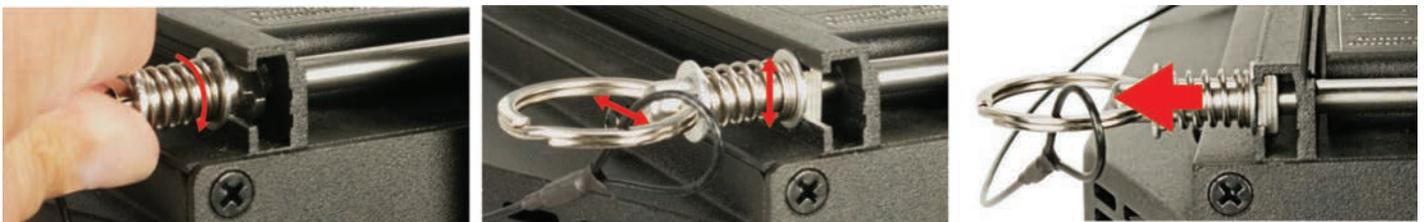
2. Compress spring and turn locking pin 90° (either direction) to lock pin into the rail. As the rail-block of the spring-loaded locking pin is stepped, it will snap the lock into place in a horizontal orientation.
