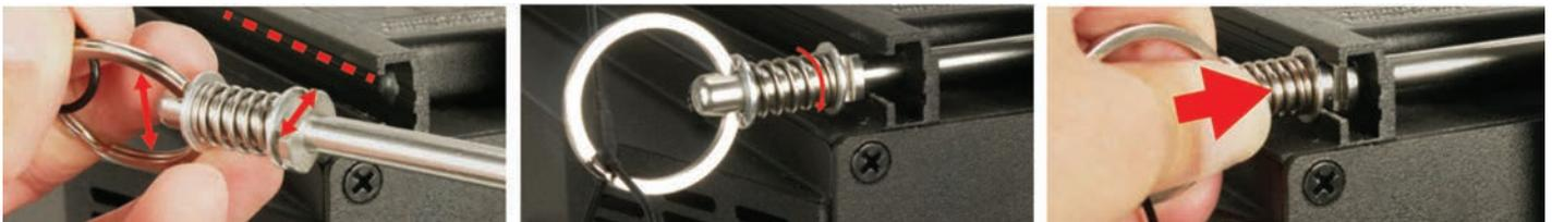
1. The spring-loaded locking pin has a stepped rail block with two flat surfaces that, when horizontally aligned with the rail, allow it to pass through. Notice that the ring orientation and the flat surfaces of the stepped rail block are perpendicular to each other.
