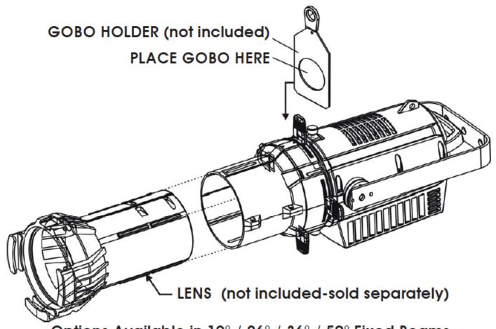
Options Available in 19 $^{\circ}$  / 26 $^{\circ}$  / 36 $^{\circ}$  / 50 $^{\circ}$  Fixed Beams
