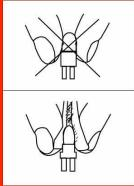
This fixture is fitted with a DISCHARGE LAMP, which is highly susceptible to damage if improperly handled. NEVER touch the lamp with your bare hands, as the oil from your hands will shorten the life of the lamp. Also, NEVER move the fixture until the lamp has had ample time to cool. Lamps are NOT covered under warranty conditions.
