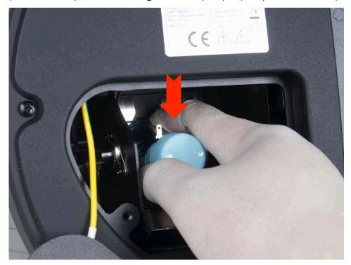
8. Gently attach the (2) Wires to spade terminals securely on the base of the lamp.
