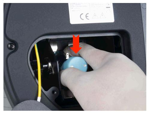
5. Once lamp is released, grab the lamp base with your thumb and index finger and gently pull the lamp **OUT** towards and **AWAY** from the fixture.
