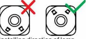
Installing direction of lamp.
