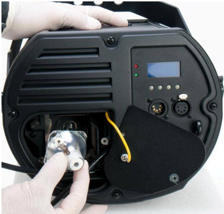
6. Using a clean cloth or gloves, gently install the new lamp into the fixture using your thumb and index finger, making sure the spade terminals on the base of the lamp are facing towards the **LEFT**.
