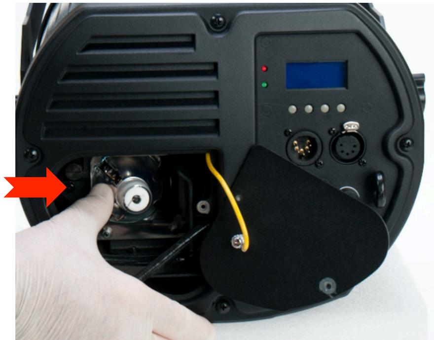
8. Make sure the lamp is properly seated into place just like the old lamp was.
