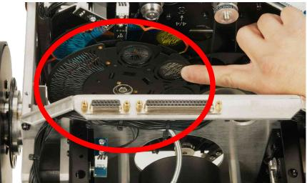
11. Carefully insert the desired Static Metal Gobos into the new Gobo/Animation wheel, making sure each of the 4 Static Metal Gobos are securely in place before installing Gobo/Animation wheel into the fixture. Reverse instructions to complete installation.
