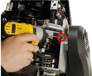
4. Remove (2x) #2 Philips screws securing the effect module.
