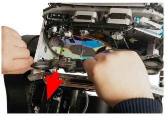
9. Because the internal lens assembly impedes the removal path of the Static Gobo wheel, disengage the TILT lock and invert the head. This will lower the internal lens assembly out and away, providing a clear path to remove the Static Gobo wheel.
