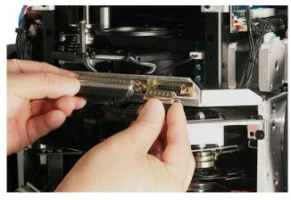
3. Remove (4x) #2 Philips screws securing 2 wire harness connectors, then carefully unplug both connectors.
