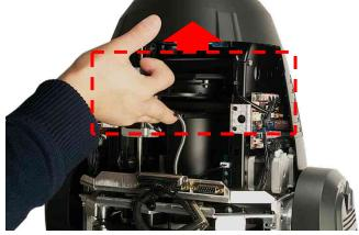
5. Because the internal lens assembly passes through the effect module tray, it needs to be lifted out and away from the effect module in order to remove it.
