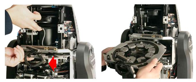
6. With the internal lens assembly lifted, carefully remove the effect module from fixture.
