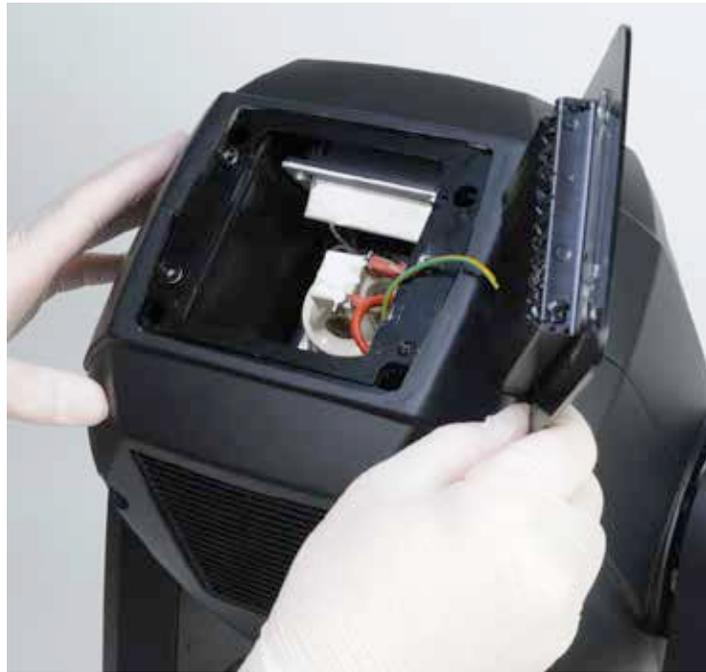
2. Using two fingers, unlock the retention clips and then gently unseat the lamp from the retention bracket and move the lamp towards you.
