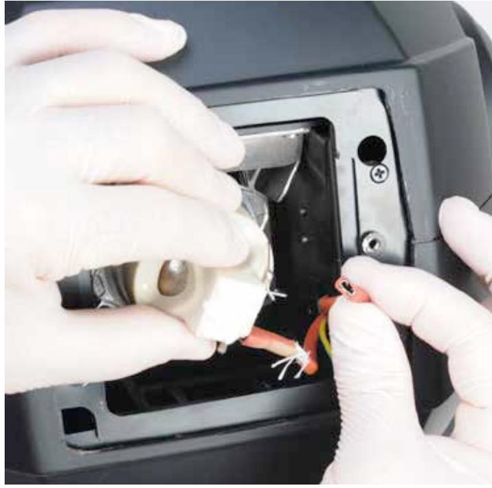
6. Gently position the new lamp into the retention bracket, making sure the lamp is seated correctly as it was before.
