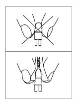
**DISCHARGE LAMP WARNING**: This fixture is fitted with a discharge lamp, which is highly susceptible to damage if improperly handled. Never touch the lamp with your bare hands, as the oil from your hands will shorten lamp life. Also, never move the fixture until the lamps have had ample time to cool. Remember, lamps are not covered under warranty conditions.
