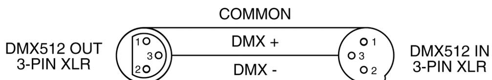
Be sure to follow the pin configuration chart below when making your own cables. Do not use the ground lug on the XLR connector. Do not connect the cable's shield conductor to the ground lug or allow the shield conductor to come in contact with the XLR's outer casing. Grounding the shield could cause a short circuit and erratic behavior.
