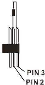
Termination reduces signal errors and avoids signal transmission problems and interference. It is always advisable to connect a DMX terminal, (Resistance 120 Ohm 1/4 W) between PIN 2 (DMX-) and PIN 3 (DMX +) of the last fixture.
