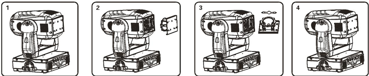
1. Set the fixture on a flat surface and remove the four screws labeled "A" "B," "C," and "D" found on the back plate of the head assembly.
