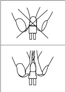
**DISCHARGE LAMP WARNING:** This fixture is fitted with a discharge lamp, which is highly susceptible to damage if improperly handled. Never touch the lamp with your bare hands, as the oil from your hands will shorten lamp life. Also, never move the fixture until the lamp has had ample time to cool. Remember, lamps are not covered under warranty conditions.
