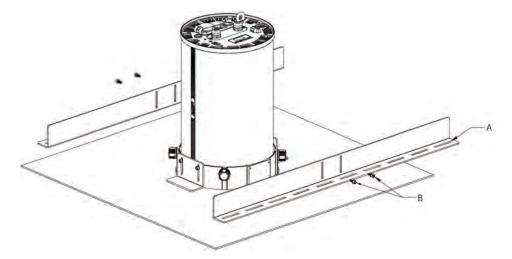
3. Attach the body support plates (A) to the trim ring using the included screws and washers (B).
