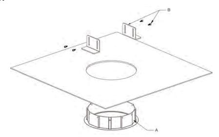
1. Open an 8.5-inch diameter hole in the desired ceiling panel. Insert the aluminum trim ring **(A)** through the hole from the underside of the panel, then secure the trim ring in place with the included screws, washers, and support brackets **(B)**.
