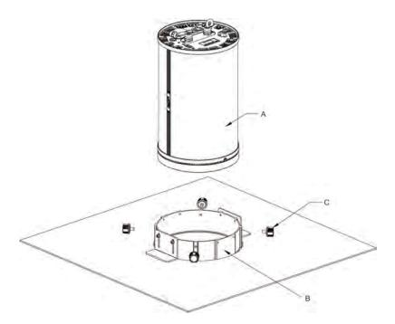
2. Lower the lighting fixture (A) into the trim ring (B) from above. Secure the lighting fixture in place by tightening the four (4) thumb screws (C).
