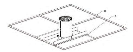
4. Install the entire assembly back into the ceiling at the desired location, making sure that the ends of the body support plates (A) are resting on firmly on the ceiling support grid (B). Secure the body support plates in place using the appropriate hardware.
