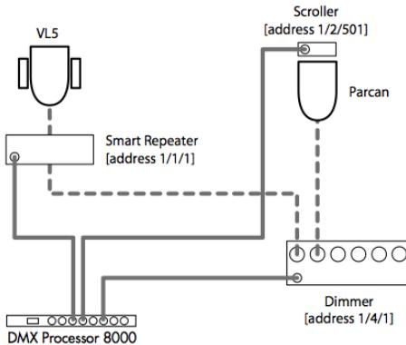
Figure 5.4. Examples of Fixtures requiring Multiple Patch Points
