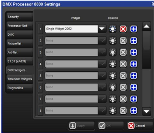
Figure 31.1. Widget Outputs pane of the DMX Processor Settings window
