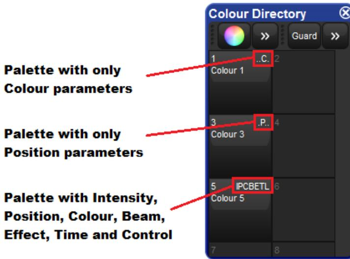
Figure 8.6. Example of Palettes containing different parameter types
