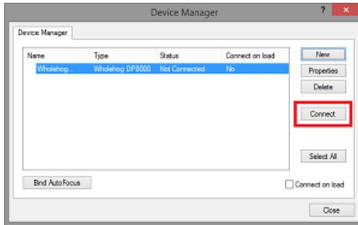
The DP8000 will now show a "connected" status which indicates that WYSIWYG is now ready to receive a visualizer data stream from a console. Please note that the "connected" status does not mean WYSIWYG is receiving a visualizer stream from a console. Proceed to *Physically Connecting the Console to the Visualizer* (p.428) for instructions on how to configure the console to send a visualizer data stream into WYSIWYG.
