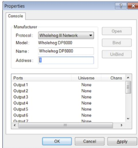
4. In the Address field enter a value of 1,2,3, or 4. If you enter a value of 1 then the output ports listed below will act as Hog visualizer outputs 1>16. If you enter an address value of 2, then the output ports displayed below will be interpreted as Hog visualizer outputs 17-32 although they are labeled output ports 1<16. Click OK to close this window.
