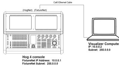
Note: In some cases it may be necessary to also right click and disable the other network adapters including bluetooth and wireless network adapters to ensure the visualizer application is sending data to the appropriate network adapter.
