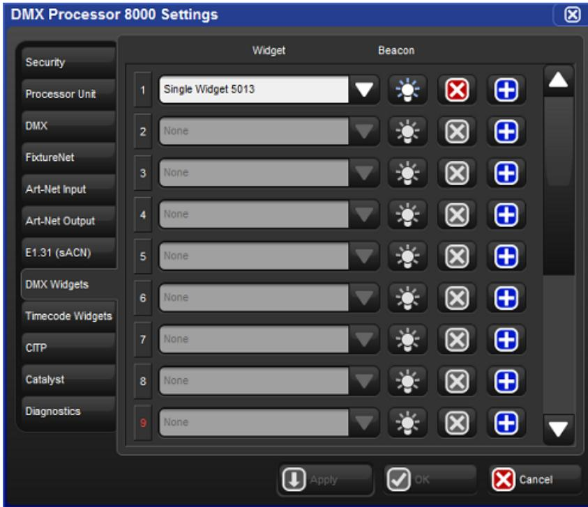
Figure 3.8. Widget Outputs pane of the DMX Processor Settings window
