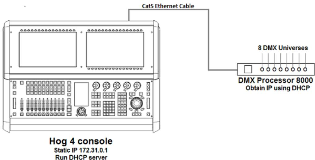
**Example B:** The console is a DHCP server, and all other nodes obtain an IP address from it.
