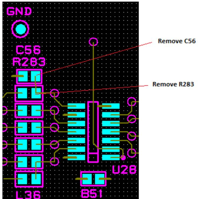
(N) Install one 330Ω 0805 resistor (HES part number 90121040EF) at reference designator R283.
