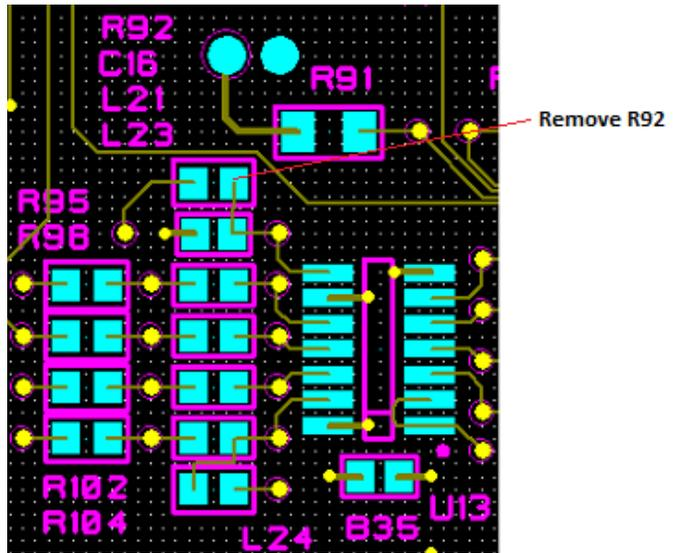
(H) Install one 330Ω 0805 resistor (HES part number 90121040EF) at reference designator R92.
