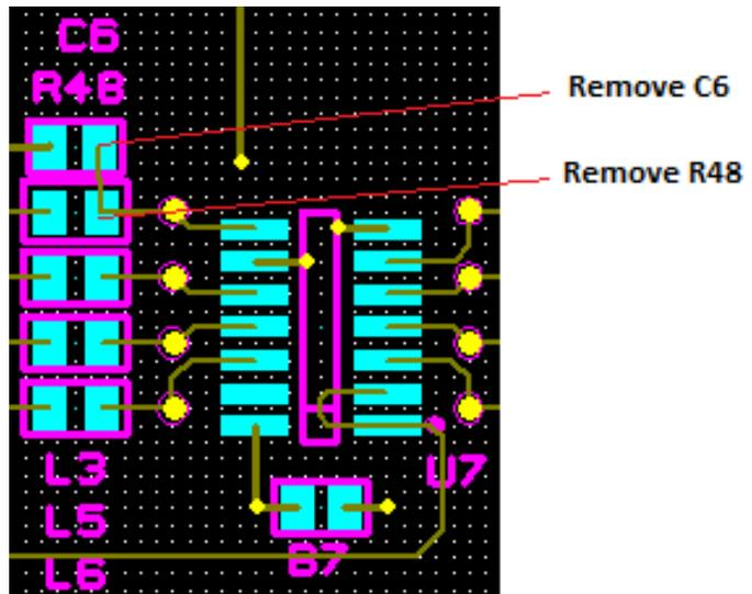
(E) Install one 330Ω 0805 resistor (HES part number 90121040EF) at reference designator R48.
