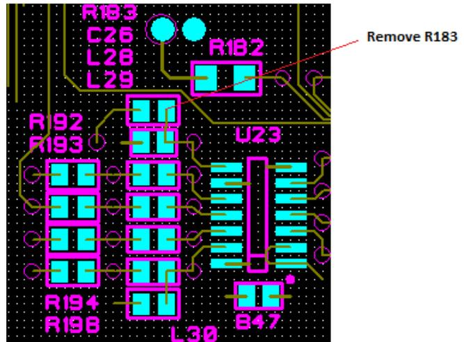
(E) Install one 330Ω 0805 resistor (HES part number 90121040EF) at reference designator R183.
