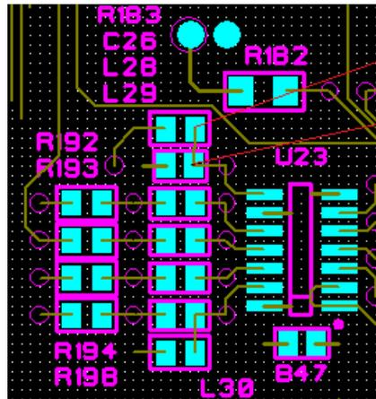
Install 330 ohm 0805 Resistor in R183 90121040EF
