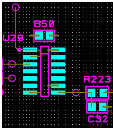
Install 330 ohm 0805 Resistor in R223 20121040EF
