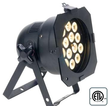
The ELED DW PAR 56 by Elation professional is a Dynamic White Prograde economical compact LED par can featuring Warm White and Cool white Tri Color LED system providing smooth white balance blending and no shadows. The ELED DW Par 56 optical system features 28 1W LED's, 14 warm white, 14 cool white -28 watts total, along with optional operating modes for stand alone or DMX control.
